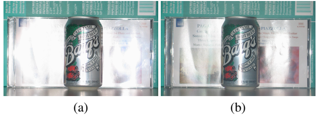
Figure 10. Shadow-free image experiment (specularities). a) Maximum of the images taken with the left and right flashes; b) shadow-free image captured with the co-located flash.
