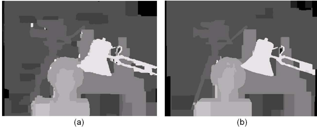
Figure 4.11: (a) Standard belief propagation result. (b) Our enhanced global stereo method, given the knowledge of depth discontinuities.
